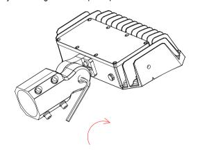
Notice: The maximum diameter of lamp pole is  $\phi$ 60, lamp adjustable angle is 0-90°.
